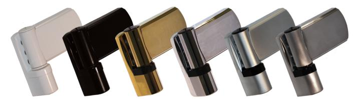
Max sash weight: 100Kg with 2 hinges Lateral adjustment: +/-5mm Height adjustment: +/-1mm Compression adjustment: +/- 0.75mm Complies with EN1935:2002 Adjustment gap cover Allows 190° opening Hinges are supplied with all covers and fixings
